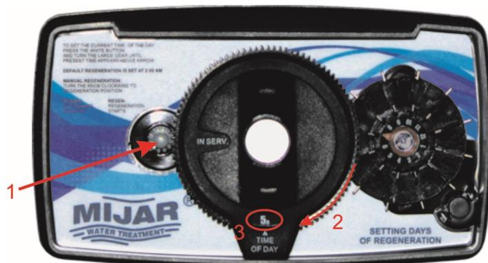
To set the current time, the user must press and hold the white button (1), and simultaneously turn the gearwheel (2) so in the gap (3) the current time is shown\* (like on the watch). Next, release the white button (1) so it falls back between the gearwheel pins.
